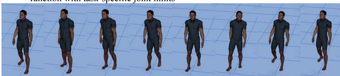
(c) Predicted motion for backward walking using joint discomfort as an objective function without task-specific joint limits
